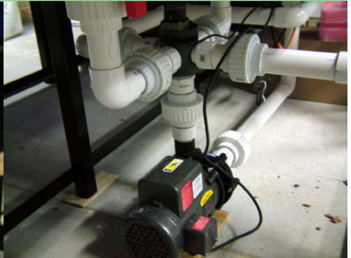
One of the Sequence® pumps plumbed to an Ocean's Motions™ 4 Way Wave-Making Device.
